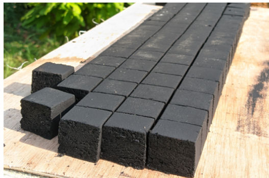
Figure 3. Briquette drying process
