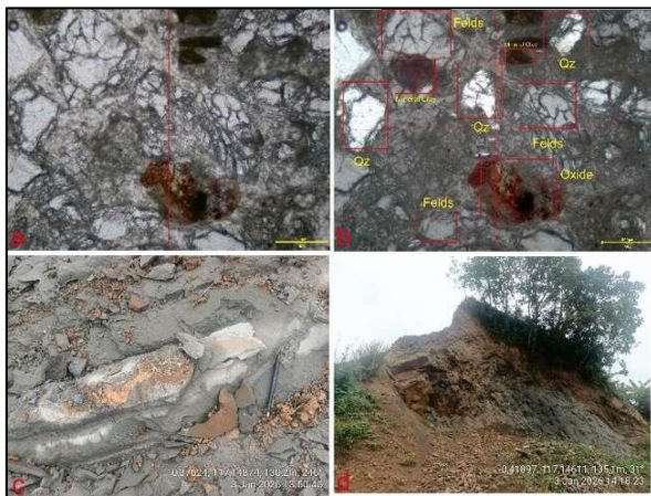
Figure 5. Explain the Appearance a. PPL Thin Incision, b. XPL Thin Incision, c. Megascopic Appearance, d. Medium Sandstone Outcrop Appearance.
