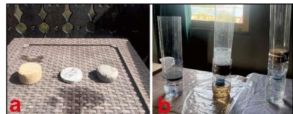
Figure 15. Explaining the Permeability Test Documentation, a. Sandstone, Limestone, and Clay Samples, b. Permeability Test Based on the Amount of Water Coming Out of Sedimentary Rock Samples.
