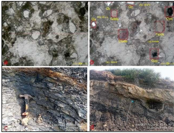
Figure 7. Explain the Appearance a. PPL Thin Incision, b. XPL Thin Incision, c. Megascopic Appearance, d. Clay Outcrop Appearance.
